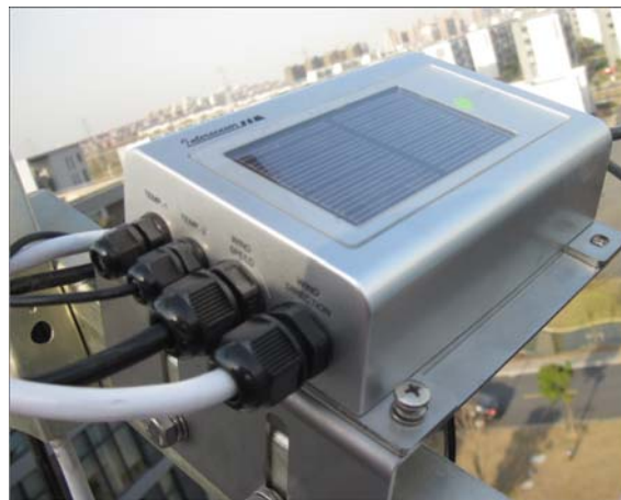
Fig 3-11 Mounting Intersensor BOX on diagonal supporting arm
