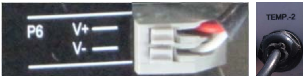
Fig 4-6 Wiring of ambient temperature sensor
